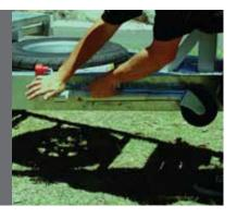
Swing up Jockey wheels must be in the horizontal position prior to towing the trailer. Never tow a trailer with the jockey wheel in the vertical position.
