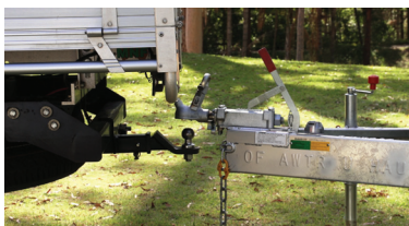
Reverse vehicle close to trailer (photo1)
