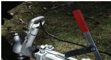
Thread lead through coupling handle (photo3)
